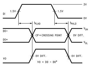
Figure 3. Driver Differential Propagation Delay Timing
