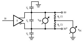
Figure 1.  $V_{\text{OD}}$  and  $V_{\text{OC}}$  Test Circuit
