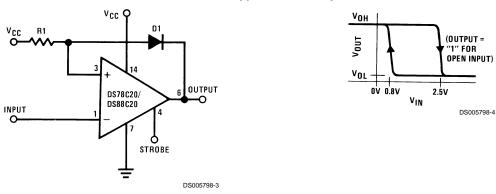
For signals which require fail-safe or have slow rise and fall times, use R1 and D1 as shown above. Otherwise, the positive input (pin 3 or 11) may be connected to ground.
