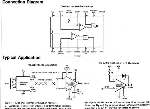
a) Capacitor in series with internal line termination resistor; terminates the line and saves termination power. Exact value depends on line length.
