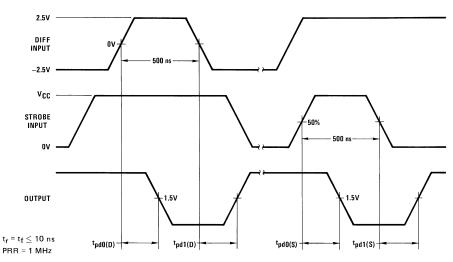
**Note**: Optimum switching response is obtained by minimizing stray capacitance on Response Control pin (no external connection).
