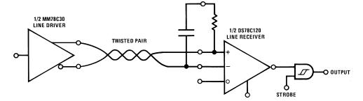
Figure 3. Balanced Data Transmission
