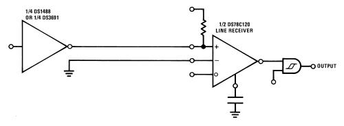
Figure 4. Unbalanced Data Transmission
