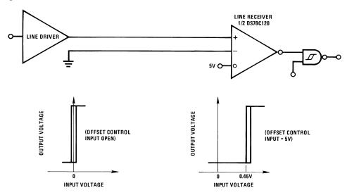
Figure 8. Unbalanced RS-423 and RS-232 Fail-Safe
