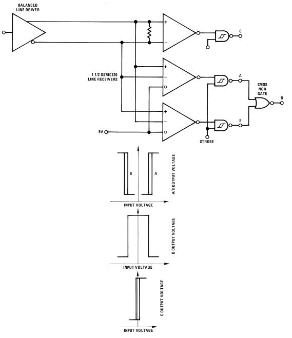
Figure 9. Balanced RS-422 Fail Safe
