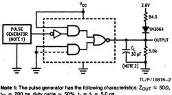
$t_{W} = 200$  ns, duty cycle = 50%,  $t_{F} = t_{F} = 5.0$  ns. Note 2: C<sub>L</sub> includes probe and jig capacitance.
