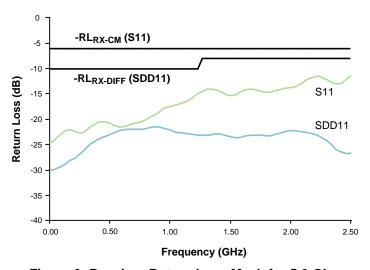
Figure 9. Receiver Return Loss Mask for 5.0 Gbps
