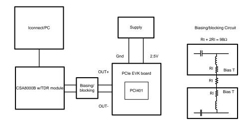
Figure 6. Input and Output Return Loss Setup
