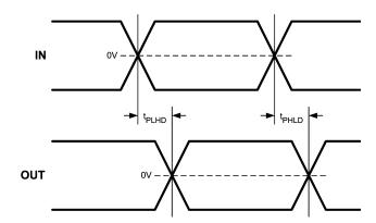
Figure 4. Propagation Delay Timing Diagram
