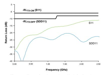
Figure 10. Transmitter Return Loss Mask for 5.0 Gbps
