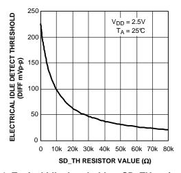
Figure 1. Typical Idle threshold vs SD\_TH resistor value
