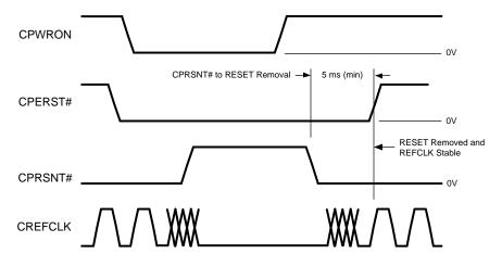
Figure 2. Typical PCIe System Timing
