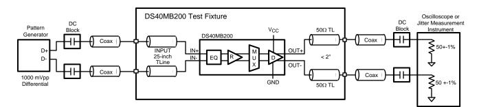
Figure 5. AC Test Circuit
