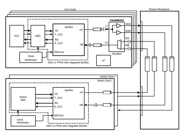
Figure 9. System Diagram (showing data paths of port 0)
