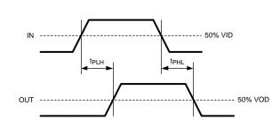
Figure 3. Propagation Delay from input to output
