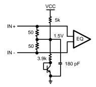
Figure 6. Receiver Input Termination and Bias Circuit
