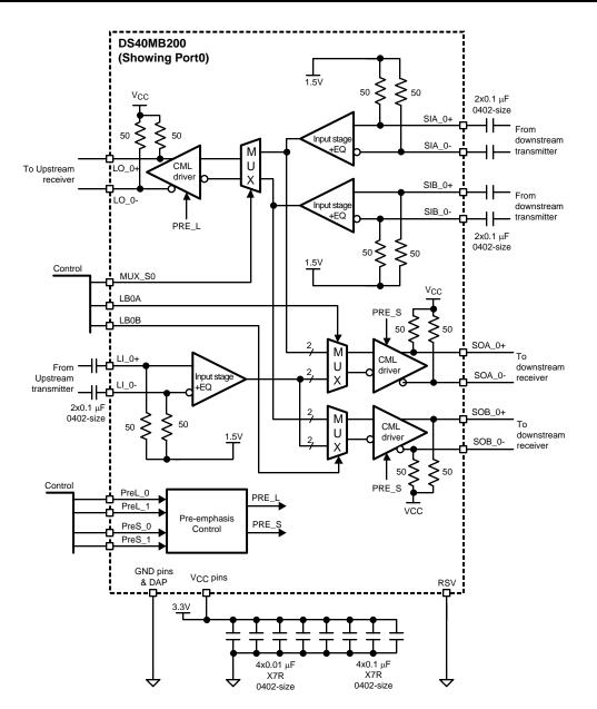
Figure 10. Application Diagram (showing data paths of port 0)
