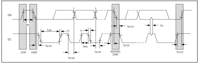
Figure 3. 2-Wire AC Characteristics
