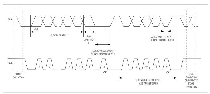
Figure 2. 2-Wire Data Transfer Protocol
