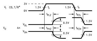
Figure 10. Receiver: CD to An,  $T/\overline{R}$  to An ( $t_{PHZ}$  and  $t_{PZH}$  only)
