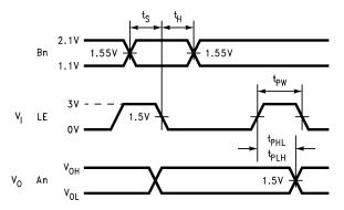
Figure 8. Receiver Enable/Disable Set-up
