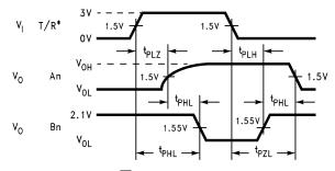
Figure 12. T/ $\overline{R}$  to Bn (t<sub>PHL</sub>and t <sub>PLH</sub> only), T/ $\overline{R}$  to An (t<sub>PZL</sub>and t <sub>PLZ</sub> only)
