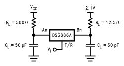
Figure 11.  $T/\overline{R}$  to An,  $T/\overline{R}$  to Bn
