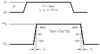
Figure 10. Driver Differential Transition Timing
