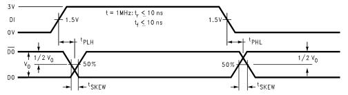
$t_{PLH}$  and  $t_{PHL}$  are measured to the respective 50% points.  $t_{SKEW}$  is the difference between propagation delays of the complementary outputs.
