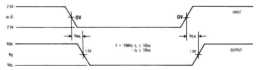
Differential input voltage may be realized by grounding RI and pulsing RI between +2.5V and -2.5V
