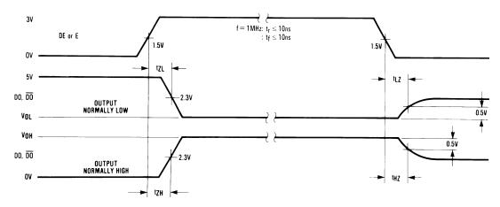
Figure 9. Driver Enable/Disable Propagation Delay Timing
