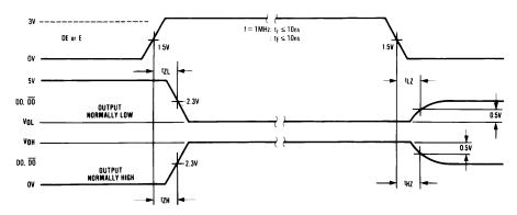
Figure 10. Driver Enable/Disable Propagation Delay Timing
