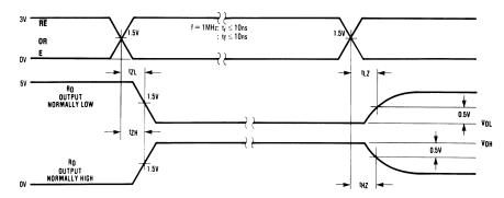
Figure 7. Receiver Enable/Disable Propagation Delay Timing
