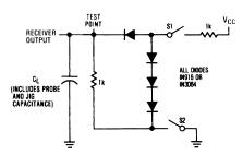
Figure 5. Receiver Propagation Delay Test Circuit
