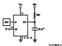
\*Includes probe and jig capacitance
