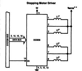
\*L1, L2, L3, L4 are the windings of a bifilar stepping motor
