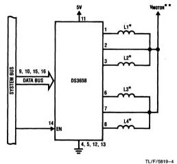
\*L1, L2, L3, L4 are the windings of a bifilar stepping motor
