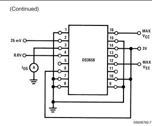
Note: Channel A shown under test, other channels are tested similarly. Only one output shorted at a time.
