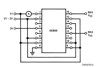
Note: Channel A(–) shown under test, other channels are tested similarly. Devices are tested with V1 from 3V to -3V.
