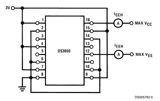
FIGURE 2. I<sub>CCH</sub> and I<sub>EEH</sub>
