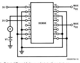
Note: Output of Channel A shown under test, other outputs are tested similarly for V1 = 0.4V and 2.4V.
