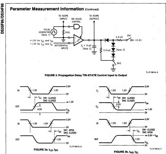
Note 1: The input pulse is supplied by a generator having the following characteristics: PRR = 1.0 MHz, 50% duty cycle,  $t_{TLH} = t_{THL} = 6.0$  ns (10% to 90%),  $Z_O = 50\Omega$ .
