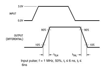
Figure 6. Differential Rise and Fall Times
