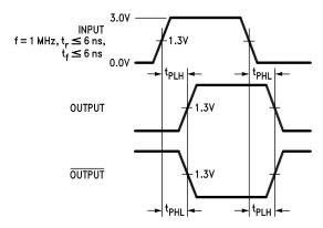
Figure 4. Propagation Delays
