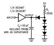
Figure 7. Propagation Delays Test Circuit for "LS-Type" Load
