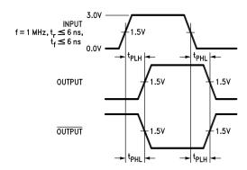
Figure 10. Load Propagation Delays for "LS-Type" Load
