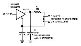
Figure 8. Differential Rise and Fall Times Test Circuit for "LS-Type" Load
