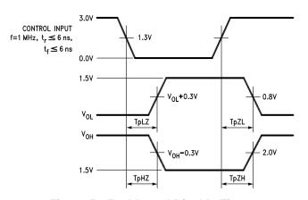
Figure 5. Enable and Disable Times
