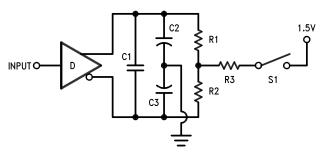
Note: C1 = C2 = C3 = 40 pF (including Probe and Jig Capacitance), R1 = R2 =  $50\Omega$ , R3 =  $500\Omega$
