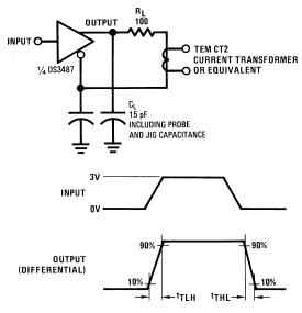
Input pulse: f = MHz, 50%;  $t_r = t_f \le 15 \text{ ns.}$
