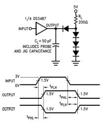
Input pulse: f = MHz, 50%;  $t_r = t_f \le 15$  ns.
