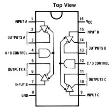
Figure 2. PDIP Package See Package Number D0016A or NFG0016E
