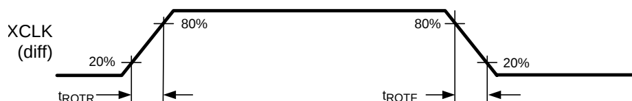
Figure 4. LVDS Output Transition Time
