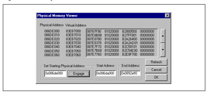
The physical memory viewer shows all the data within the start and end address space that is allocated by the BoSS program. The user can step through memory by the address box or the scroll up/down buttons on the right.
