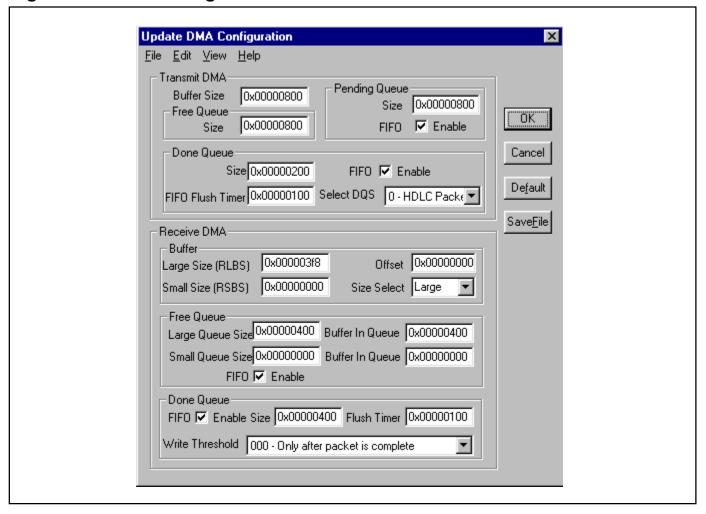
The DMA configuration displays default values at first, then the user can change the desired value and hit the Master Reset. The DMA in BoSS can read from as well as write to the receive free queue and transmit pending queue. Therefore, each access of the descriptor queues are done one at a time, and sequentially.
