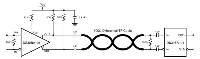
Figure 2. Cable Extender Chipset Application Circuit for 100Ω Differential Cable
