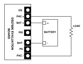
Fig 2b: Discharging Circuit
