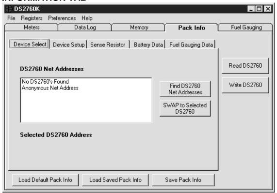
The Pack Information tab gives the pack manufacturer the ability to assign default register settings, device and sense resistor selection, and recommended manufacturer data and fuel gauging information.
