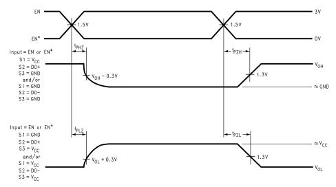
Figure 6. Driver Single-Ended TRI-STATE Waveforms
