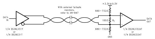
Figure 7. Typical Driver Connection
