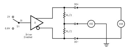
Figure 2. Differential Driver DC Test Circuit
