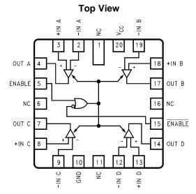
Figure 2. 20-Lead LCCC Package See Package Number NAJ0020A
