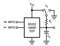
$\ensuremath{\mathsf{C}}_{\ensuremath{\mathsf{L}}}$  includes load and test jig capacitance.
