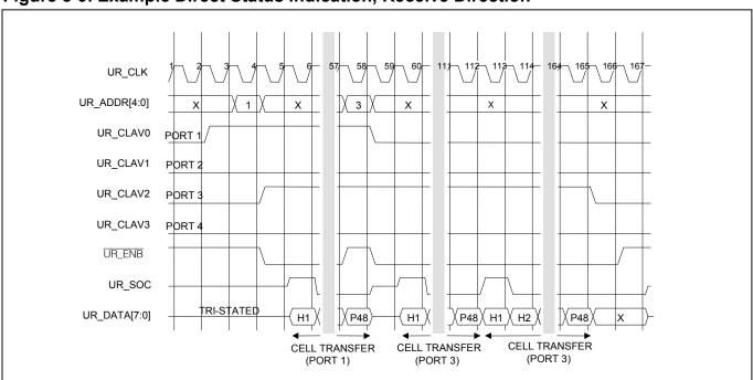
Figure 8-9. Example Direct Status Indication, Receive Direction
