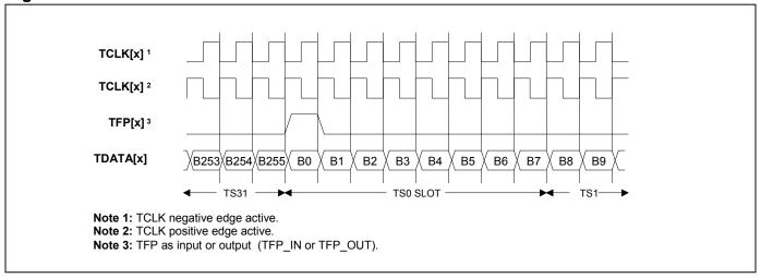
Figure 7-9 shows the transmit framer-interface operation for E1 in gapped-clock mode.
