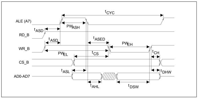
Figure 13-3.Motorola Bus Timing (BTS = 1/MUX = 1)
