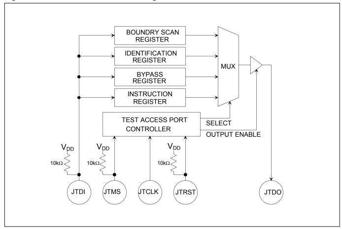
**TAP Controller State Machine.** The TAP controller is a finite state machine that responds to the logic level at JTMS on the rising edge of JTCLK (<u>Figure 11-2</u>).
