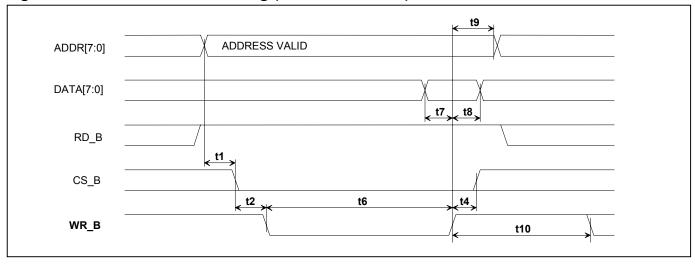
Figure 13-6. Motorola Bus Read Timing (BTS = 1/MUX = 0)
