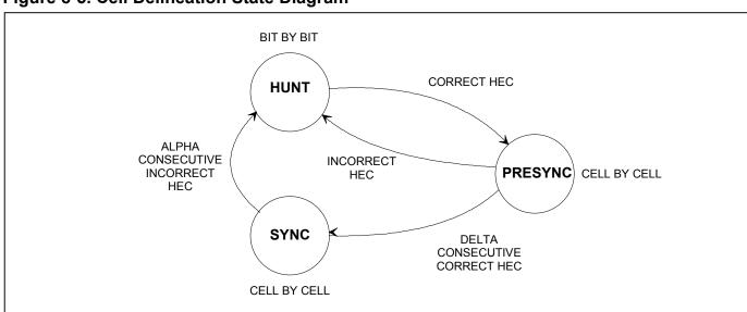
Figure 8-5. Cell Delineation State Diagram
