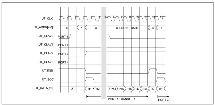
Figure 7-4. Example of Direct Status Indication, Transmit Direction
