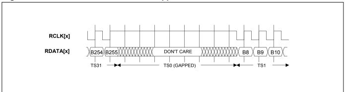
The fractional T1 (N x DS0) is supported in RFP and gapped-clock modes of physical interface. In RFP mode, the framer must generate RFP during frame-overhead-bit and nonactive-DS0-channel positions. In gapped-clock mode, RCLK should be gapped during frame-overhead-bit and nonactive-DS0-channel positions. In E1 mode, the DS26101 should be configured in gapped-clock mode and RCLK should be gapped during nonactive time slots. **RFP mode is not supported in fractional E1 configuration.**
