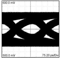
Figure 23. A 2.5 Gbps NRZ PRBS-23 without PE After 30" Differential FR-4 Stripline H: 75 ps / DIV, V: 100 mV / DIV
