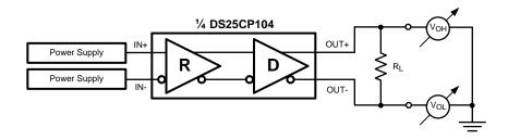
Figure 1. Differential Driver DC Test Circuit
