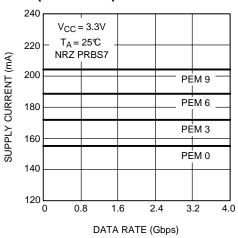
Figure 22. Supply Current as a Function of Data Rate and PE Level
