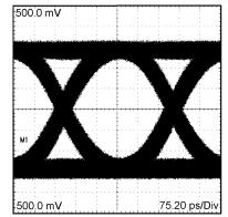
Figure 25. A 2.5 Gbps NRZ PRBS-23 with High PE After 30" Differential FR-4 Stripline H: 75 ps / DIV, V: 100 mV / DIV
