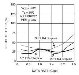
Figure 19. Residual Jitter as a Function of Data Rate, FR4 Stripline Length and PE Level
