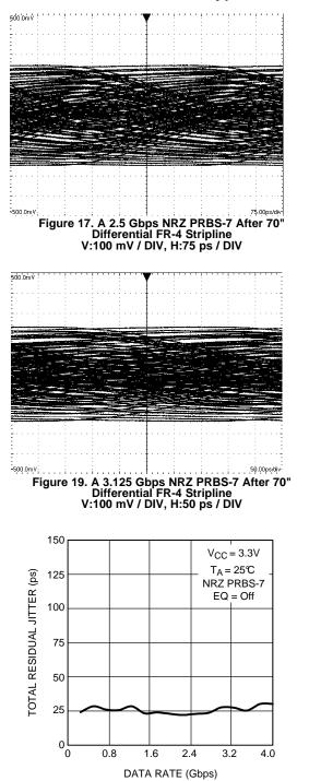
Figure 21. Total Jitter as a Function of Data Rate
