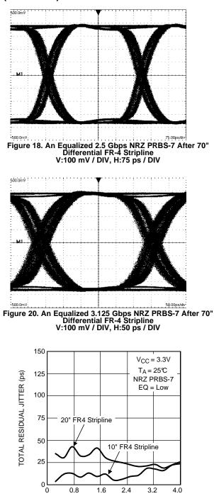
Figure 22. Total Jitter as a Function of Data Rate
