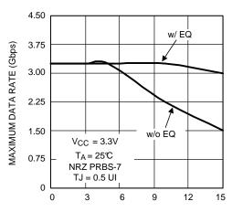
CAT5e LENGTH (m) Figure 12. Maximum Data Rate as a Function of CAT5e (Belden 1700A) Length
