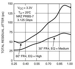
DIFFERENTIAL INPUT VOLTAGE (V) Figure 28. Total Jitter as a Function of Input Amplitude
