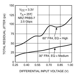
Figure 26. Total Jitter as a Function of Input Amplitude
