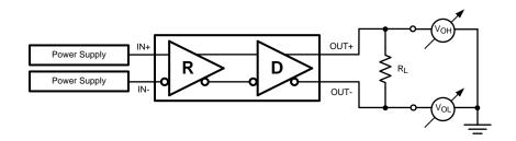
Figure 1. Differential Driver DC Test Circuit
