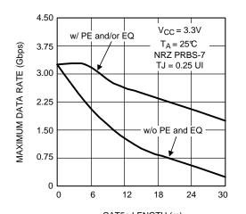
CAT5e LENGTH (m) Figure 13. Maximum Data Rate as a Function of CAT5e (Belden 1700A) Length DS25BR120 Used as a Driver DS25BR110 Used as a Receiver
