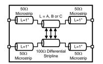
Figure 6. Test Channel Description
