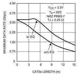
Figure 11. Maximum Data Rate as a Function of CAT5e (Belden 1700A) Length
