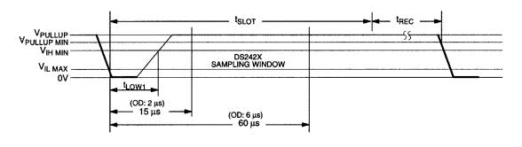
Regular Speed 60  $\mu$ s  $\leq$  t<sub>SLOT</sub> < 120  $\mu$ s 1  $\mu$ s  $\leq$  t<sub>LOW1</sub> < 15  $\mu$ s 1  $\mu$ s  $\leq$  t<sub>REC</sub> <  $\infty$
