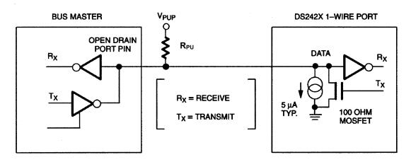
Note: Depending on the 1-Wire communication speed and the bus load characteristics, the optimal pull-up resistor ( $R_{PU}$ ) value will be in the 1.5k $\Omega$  to 5k $\Omega$  range.
