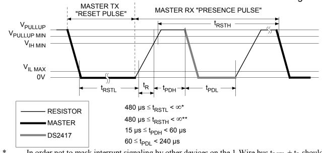
**INITIALIZATION PROCEDURE "RESET AND PRESENCE PULSES"** Figure 8
