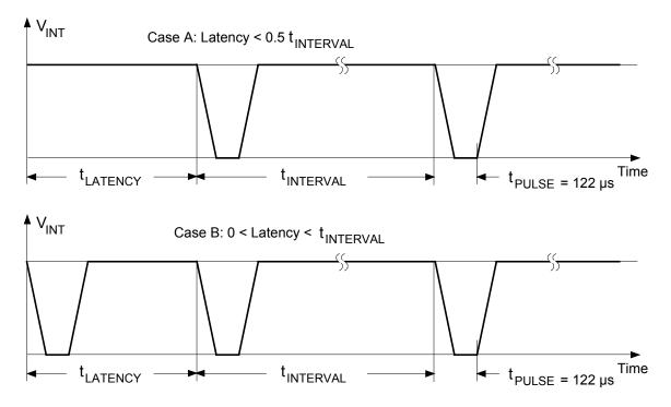
The latency depends on the selected interrupt interval (IS0 to IS2 settings) and the contents of the RTC counter at the time of writing the device control byte. In Case A, the flip-flop that determines the interval duration is reset and toggles before half of the interval time is over. In Case B, this flip-flop is set that generates an immediate interrupt pulse; the latency, therefore, can be up to one full interval duration.
