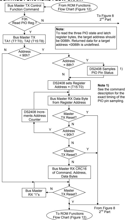
Figure 8-2. CONTROL FUNCTIONS FLOW CHART
