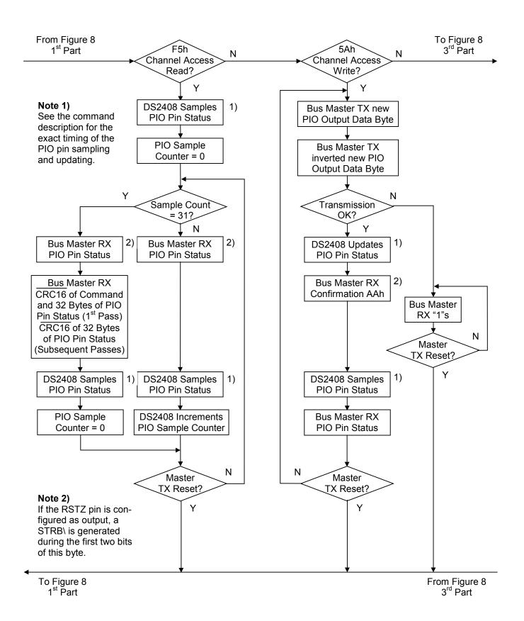
Figure 8-3. CONTROL FUNCTIONS FLOW CHART
