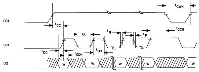
3-WIRE READ DATA TIMING DIAGRAM Figure 20
