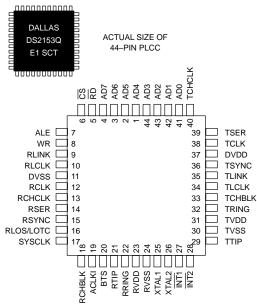
The DS2153 automatically adjusts to E1 22 AWG (0.6 mm) twisted—pair cables from 0 to 1.5 KM. The device can generate the necessary G.703 waveshapes for both 75 ohm and 120 ohm cables. The onboard litter
