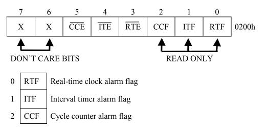
When a given alarm occurs, the corresponding alarm flag is set to a logic 1. The alarm flag is cleared by reading the status register.
