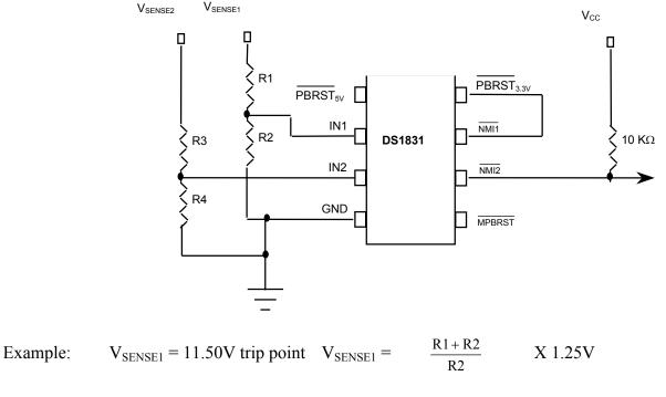
Therefore:  $11.50V = \frac{R1 + 100 k\Omega}{100 k\Omega} \times 1.25V$
