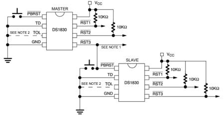
**Note 1:** The RST3 output tied to the pushbutton reset would be pulled to  $V_{CC}$  through the 40KW resistor in the pushbutton input. If a stronger pull-up is required an additional pull-up resistor could be added.
