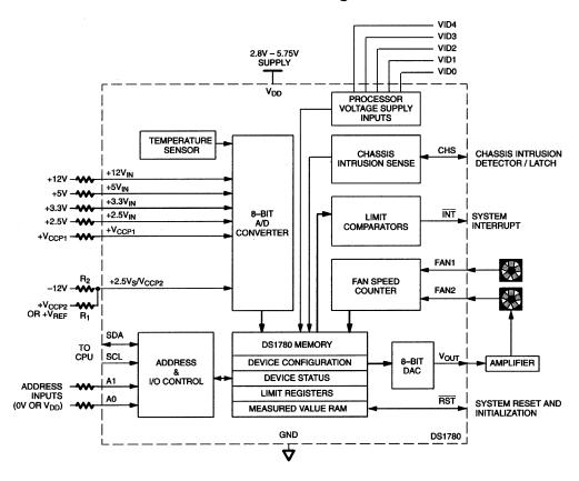
**Note:** R1 and R2 on the -12V resistance ladder should be ratioed such that approximately +2.5V appears at the input pin (i.e., R1=4k $\Omega$ , R2=23.2 k $\Omega$ ). If a second processor voltage needs to be monitored (V<sub>CCP2</sub>), leave R2 empty, and make R1 500 $\Omega$ , with V<sub>CCP2</sub> appearing here.
