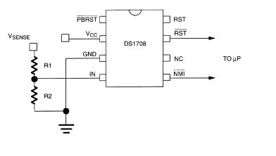
$$V_{\text{SENSE}} = \frac{R1+R2}{R2} X 1.25 \qquad \qquad V_{\text{MAX}} = \frac{V_{\text{SENSE}}}{V_{\text{TP}}} X V_{\text{CC}}$$
