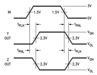
Figure 4. Driver Propagation Times (2)(4)
