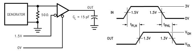
Figure 7. Receiver Propagation Delay Times (5)(6)
