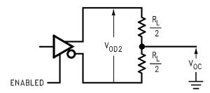
Figure 1. Driver  $V_{OD}$  and  $V_{OC}^{(1)}$
