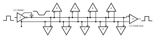
Figure 10. Fully Loaded RS-423 Interface
