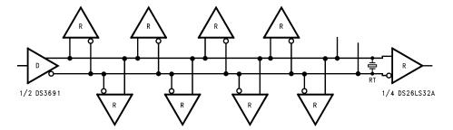
Figure 8. Fully Loaded RS-422 Interface
