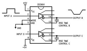
Figure 12. Dual RS-423 Inverting Driver
