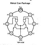
Pin 4 is in electrical contact with the case
