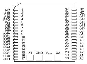
34-Pin PowerCap Module Board (Uses DS9034PCX PowerCap)
