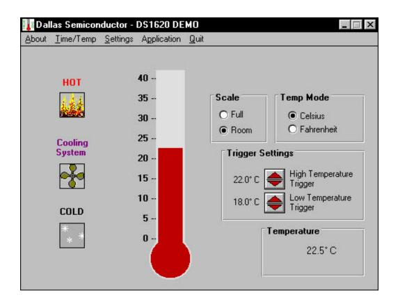
The DS1620K demonstration kit allows a potential user of the DS1620 to observe the operation of the DS1620 in an actual temperature measurement application. Temperature is measured and displayed in a text box, as well as on a graphical thermometer. Thermostat trip-points may be set by the user, and a graphical display of the status of each thermostat output is available on the screen at all times. Temperature may be displayed in Celsius or Fahrenheit.
