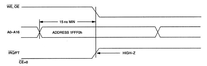
The  $\overline{IRQ}/FT$  pin can also be activated in the battery backed mode. The  $\overline{IRQ}/FT$  will go low if an alarm occurs and both ABE and AE are set. The ABE and AE bits are cleared during the power-up transition, however an alarm generated during power-up will set AF. Therefore the AF bit can be read after system power-up to determine if an alarm was generated during the power-up sequence. Figure 4 illustrates alarm timing during the battery back-up mode and power-up states.
