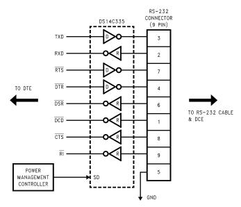
Figure 10. Typical DTE Application
