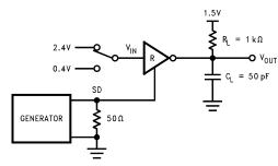
Figure 8. Receiver SHUTDOWN (SD) Delay Test Circuit
