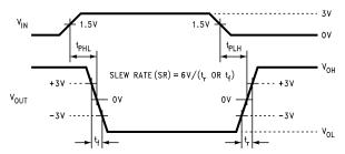
Figure 3. Driver Propagation Delay and Slew Rate Timing
