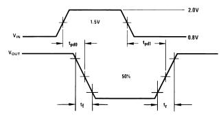
$t_{\rm r}$  and  $t_{\rm f}$  are measured between 10% and 90% of the output waveform.
