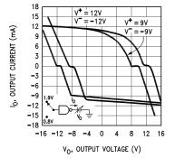
Figure 10. Output Voltage and Current-Limiting Characteristics
