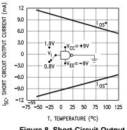
Figure 8. Short-Circuit Output Current vs Temperature
