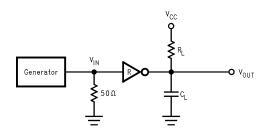
Figure 4. Receiver Propagation Delay and Transition Time Test Circuit <sup>(6)</sup>
