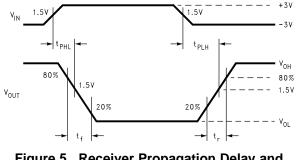
Figure 5. Receiver Propagation Delay and **Transition Time Waveform**
