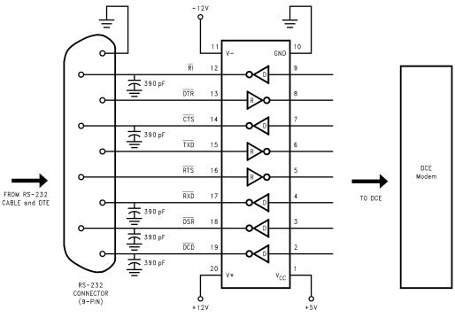
Figure 9. Typical DCE Application
