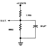
\*INCLUDING SCOPE AND JIG CAPACITANCE
