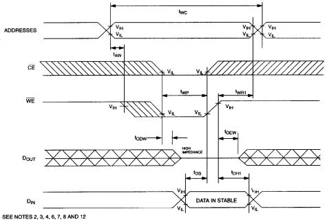
**TIMING DIAGRAM: WRITE CYCLE 2**
