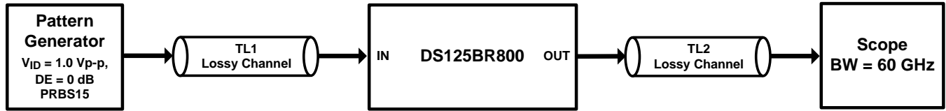
Figure 23. Test Setup Connections Diagram
